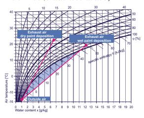
Higher exhaust air moisture produces more condensed water and excess water in the rotor.
