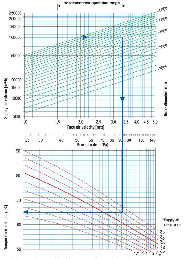
The design program for rotor profile A25 is most commonly used in paint spraying systems. Air flows relate to standard density of  $\rho=1.20~kg/m^3$
