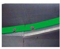
Permanently fixed plastic seals or profiled sheet metal with extremely small clearance to the rotor are used as center seals.
