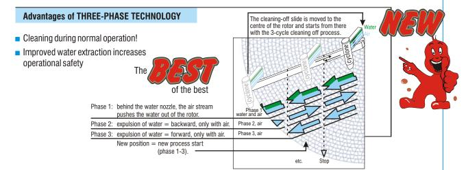
With THREE-PHASE TECHNOLOGY rotors can be excellent cleaned during operation of the ventilation plant.
